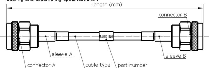
Corrugated cables available (flexible, superflexible and extraflexible) and specifications comparator :  $\underline{PDF}$
